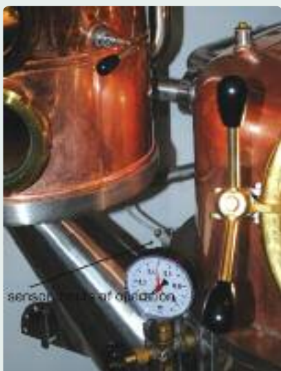
Right: Annotated photograph of the excise metering on the still. Below: The position of the sensor recording the hours of operation. Below centre: The flow sensor. Below right: The 'how often filled' sensor on top of the pot still.
